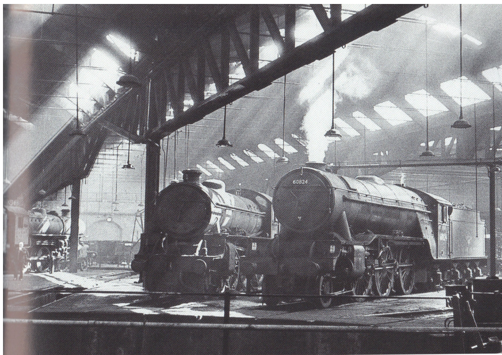
YORK: Dated 1 May 1966, this interior shot of York North shed illustrates so vividly the atmosphere of a roundhouse. From left to right are a BR Standard 4MT 2-6-0, a 'B1' 4-6-0 and ex-LNER 'V2' 2-6-2 No 60824 with a 34A shedplate (St Margaret's, Edinburgh).
